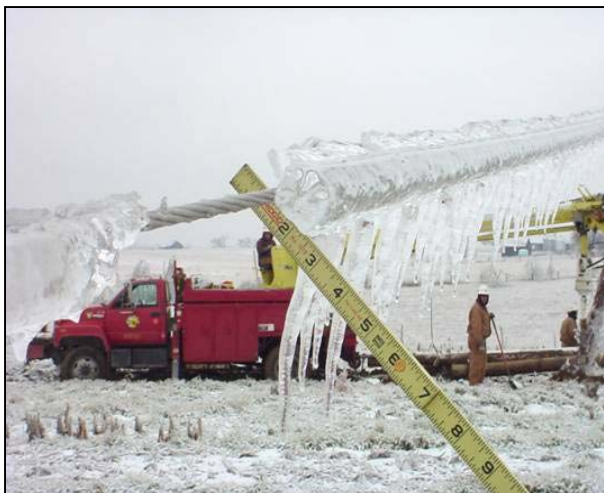
PHOTO 34: Ice Accumulation on #2ACSR Wire Near Lexington, KY
