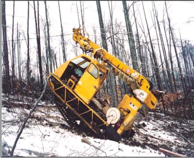
PHOTO 15: “All-Terrain” Tracked Digger-Derrick
